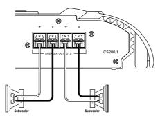
**Figure 2.** CS subwoofer amplifier with two woofer connections.
